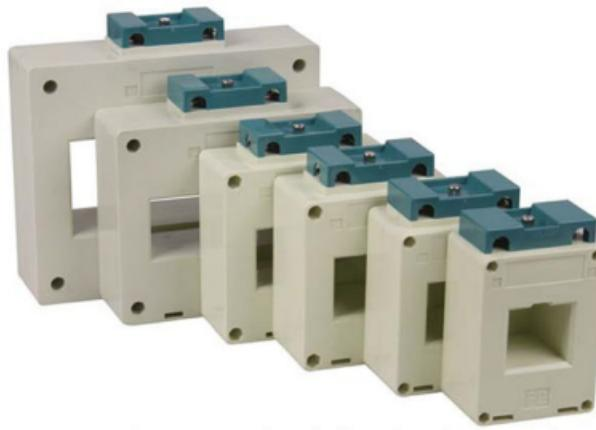
CTBHII series low-voltage current transformers are mainly used in low-voltage distribution cabinets to transform the current of cables or copper bars. The general CTBHII series products are used on copper bars, and the current transformers are directly fixed on the copper bars using the fixed accessories provided, which is convenient and flexible.
